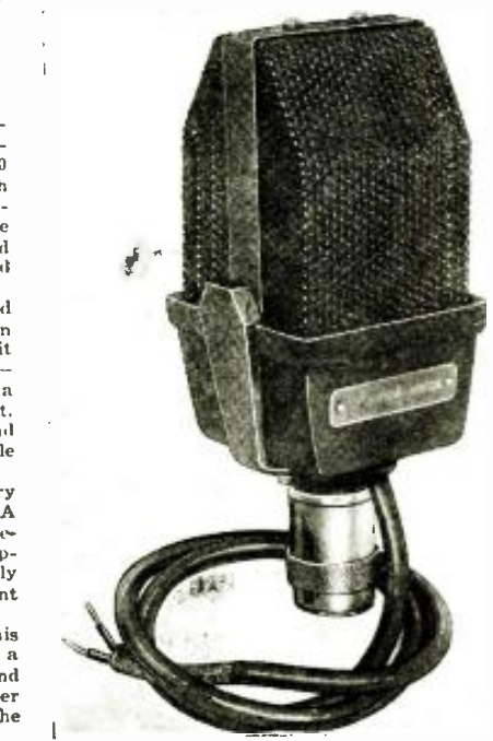
Fig. A. A view of the completed ribbon microphone.
