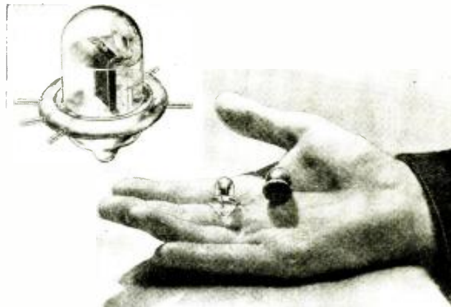
Fig. A. Physical comparison of the new "955" tube with an acorn.
