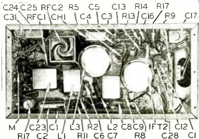
Fig. D, below. Underside view of chassis and layout. Refer to List of Parts for interpretation of various symbols and values.
